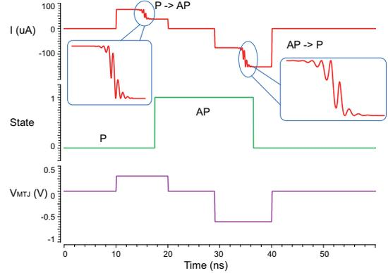
**Figure 3: The transition of electrical parameters during the switching process of MTJ under voltage pulses. The oscillation is induced by the precessional motion of perpendicular anisotropy filed.**
