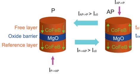
**Figure 1: Typical structure of PMA-MTJ.**
