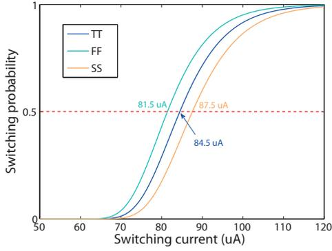
**Figure 5: Switching probability of MTJs on function of switching current with 10ns pulse. The current with 50% switching success is indicated above. This figure is obtained by 1000 runs of Monte-Carlo simulation with the same MTJ under voltage pulses.**
