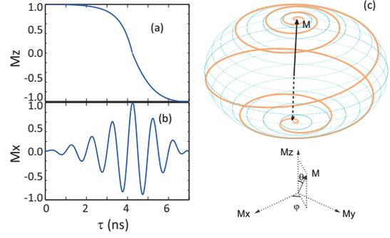
**Figure 2: The precession of magnetization under the influence of a spin current: Time dependence of (a) Mz and (b) Mx, (c) The reversal process of magnetic moment.**
