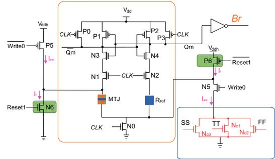
**Figure 7: MTJ writing circuit and PCSA:  $I_{sw}$  is the switching current flowing through MTJ during random writing phase and  $I_r$  is the switching current during reset phase.  $N_{c0}$ ,  $N_{c1}$  and  $N_{c2}$  modulate the switching current according to the random number probability obtained in the precedent cycle.**
