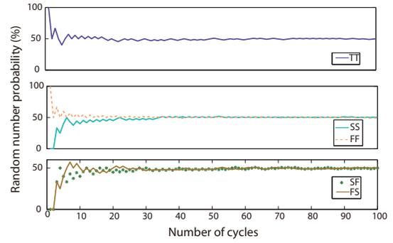
**Figure 10: Output ‘1’ probability versus number of clock cycles: The output random number probability becomes stable after 30 cycles (The probability of ‘1’ occurrence stays around 50%) for all the five corner models.**
