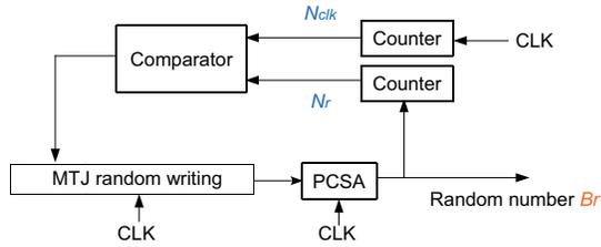
**Figure 6: Architecture of proposed MTJ-based true random number generator: The random writing circuit generates a switching current to write the MTJs with 50% success and it is controlled by the correction block; The MTJ writing part enables MTJ switching (generating random number or resetting to initial state); The correction block composed of counter and comparator is used to execute real-time output probability tracking and send feedback to writing block.**
