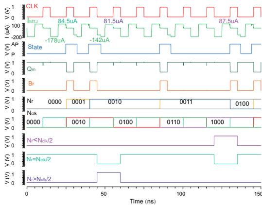
**Figure 9: Time-domain diagram of proposed true random number generator. During each cycle, the MTJs are firstly reset to the initial state (with  $I_r=178\mu A$  for P state and  $I_r=142\mu A$  for AP state), then randomly switched, and finally sensed at the output. The initial current is set for 50% of switching success.**
