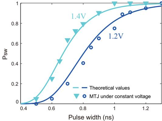
**Figure 4: Switching probability  $P_{sw}$  as a function of pulse width: the lines are theoretical values plotted from (6) and the markers are statistical results from 1000 times of Monte Carlo simulation.**
