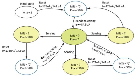
**Figure 8: The phase transition diagram of proposed circuit design: The three states in blue frame are with different output random number probability after reset phase; The state in green signifies the unknown switching probability after random writing phase; The three states in yellow are with different known random number probability after sensing phase. For MTJs, ‘0’ represents P state and the resistance is relatively low. ‘?’ represents unknown information.**
