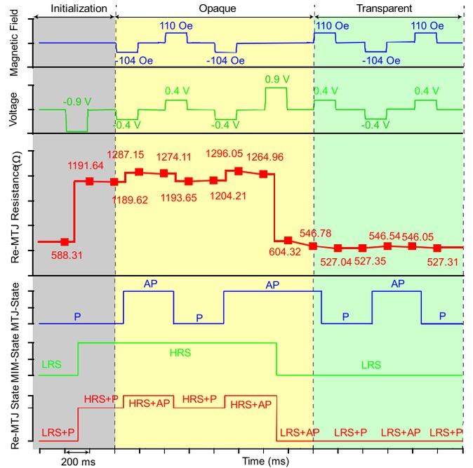
Fig. 3. Experimental demonstration of the functional behavior for memory encryption enabled by Re-MTJ device with transparent feature.
