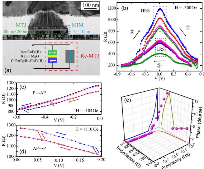
**Fig. 1.** (a) Cross-sectional HRTEM image and the corresponding device model of Re-MTJ. The Re-MTJ has a device structure of an MTJ in parallel connection with an MIM. The blue balls represent the conductive filaments; (b)–(d) Transport measurements show both the resistive switching as (b) and magnetic switching as (c) and (d); (e) AC-impedance spectroscopy of the device at 20 mV.
