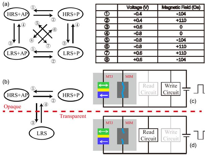
Fig. 2. The state transition diagrams of Re-MTJ device under a combination of voltage and magnetic field. (a) Four resistance states with a combination of configuration of conductive filaments (HRS or LRS) and MTJ (AP or P); (b) Three resistance states for ignoring MTJ states when the conductive filaments are on (LRS). (c) Writing and (d) reading operation of Re-MTJ device for the application as encryption memory.
